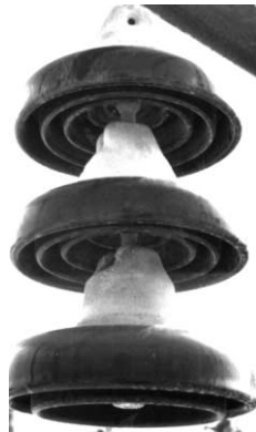
Fig. 1. The insulator string.
